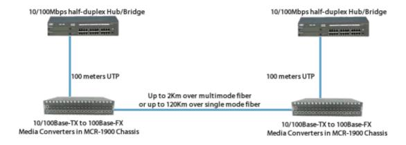
10/100 - Extend Network between Half-Duplex Hub and Switch
